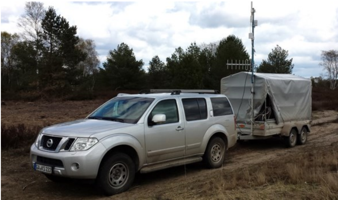
Figure 10: Workplace of the operator of the unmanned, remote-controlled caterpillar, showing wireless transmission system and trailer housing a generator. For further explanations, see text.
