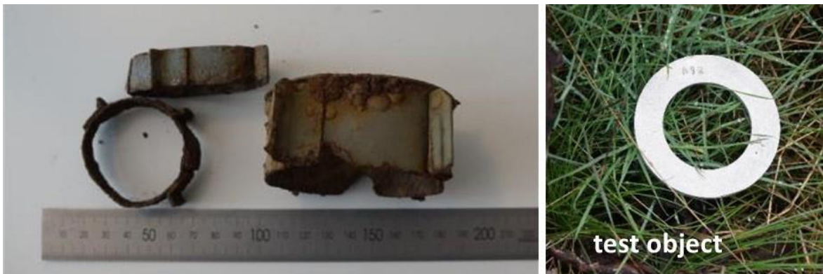
Figure 21: Objects of the minimum size to be detected (left) and a test object used to check the effectiveness of clearance work (right)
