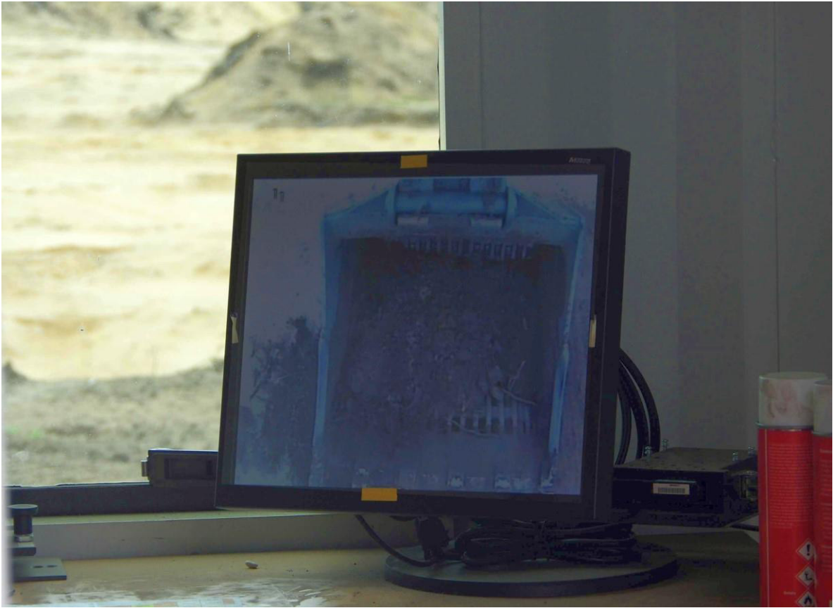
Figure 18: Video monitoring of the operation of a screening bucket
