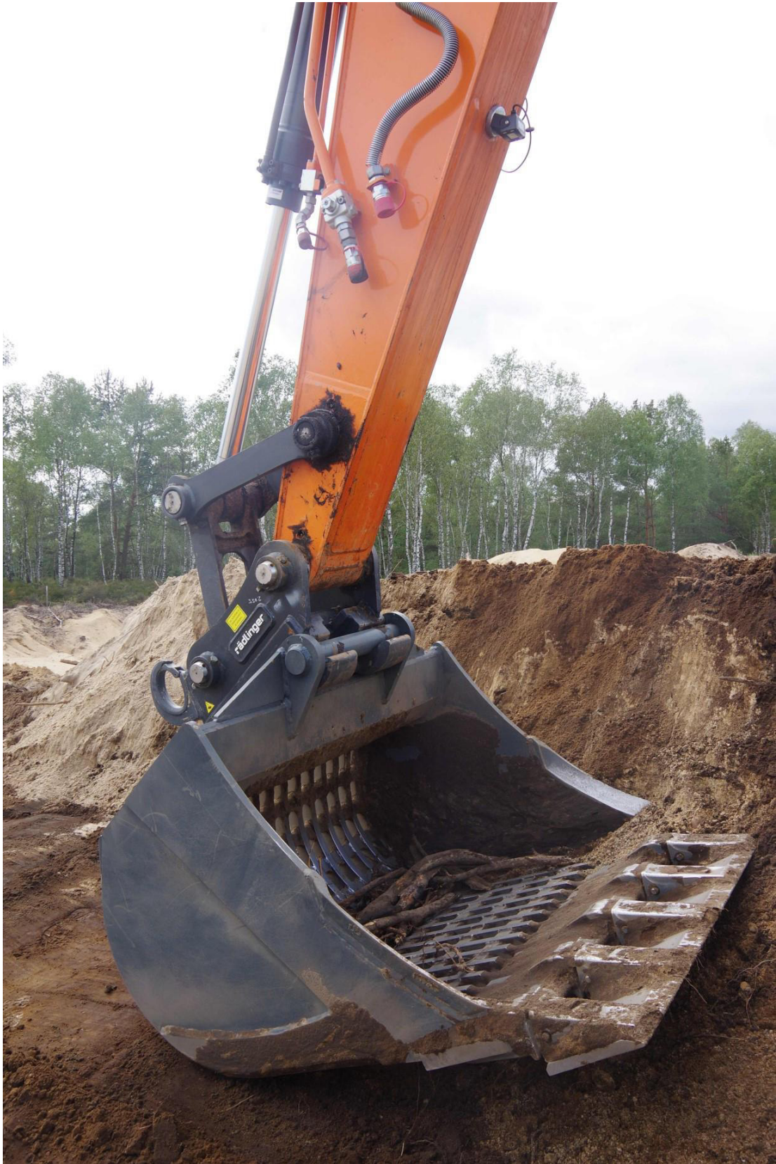
Figure 17: Screening bucket in operation. One of the monitoring cameras can be seen on the arm of the excavator.
