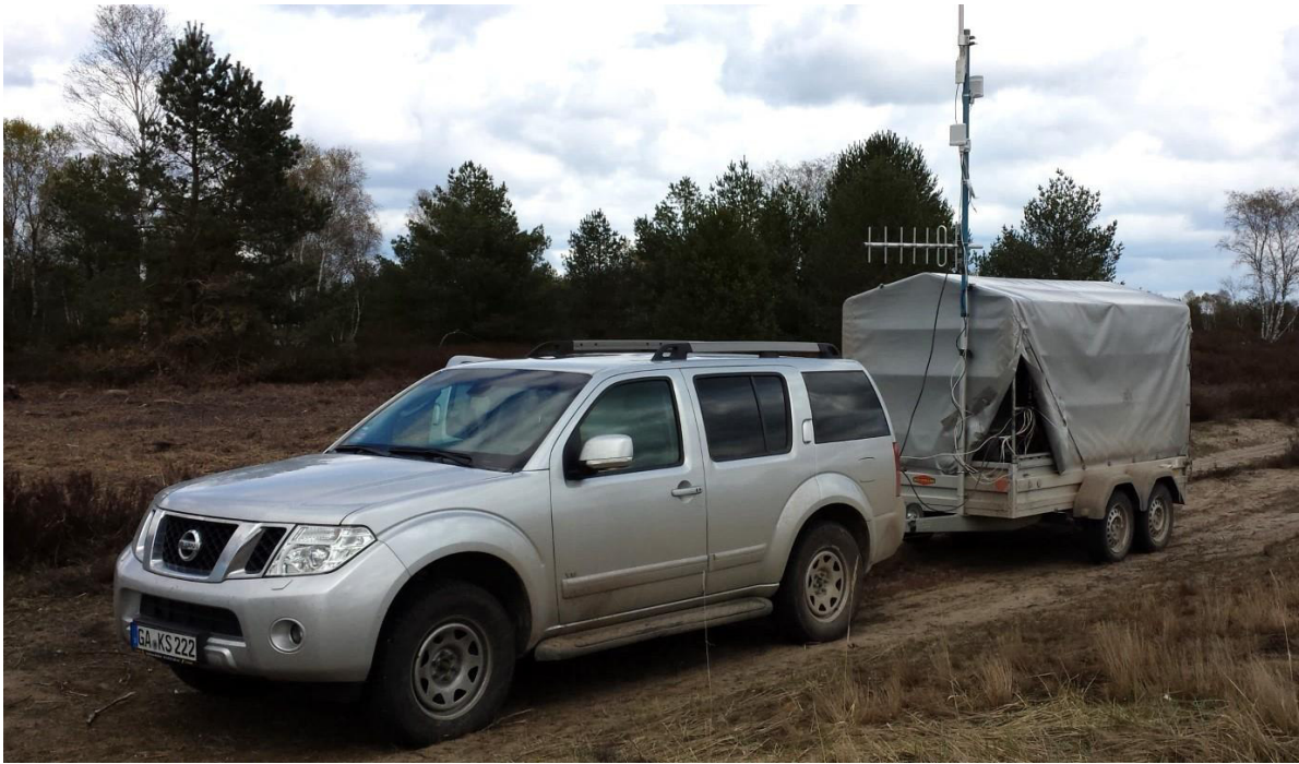
Figure 10: Workplace of the operator of the unmanned, remote-controlled caterpillar, showing wireless transmission system and trailer housing a generator. For further explanations, see text.
