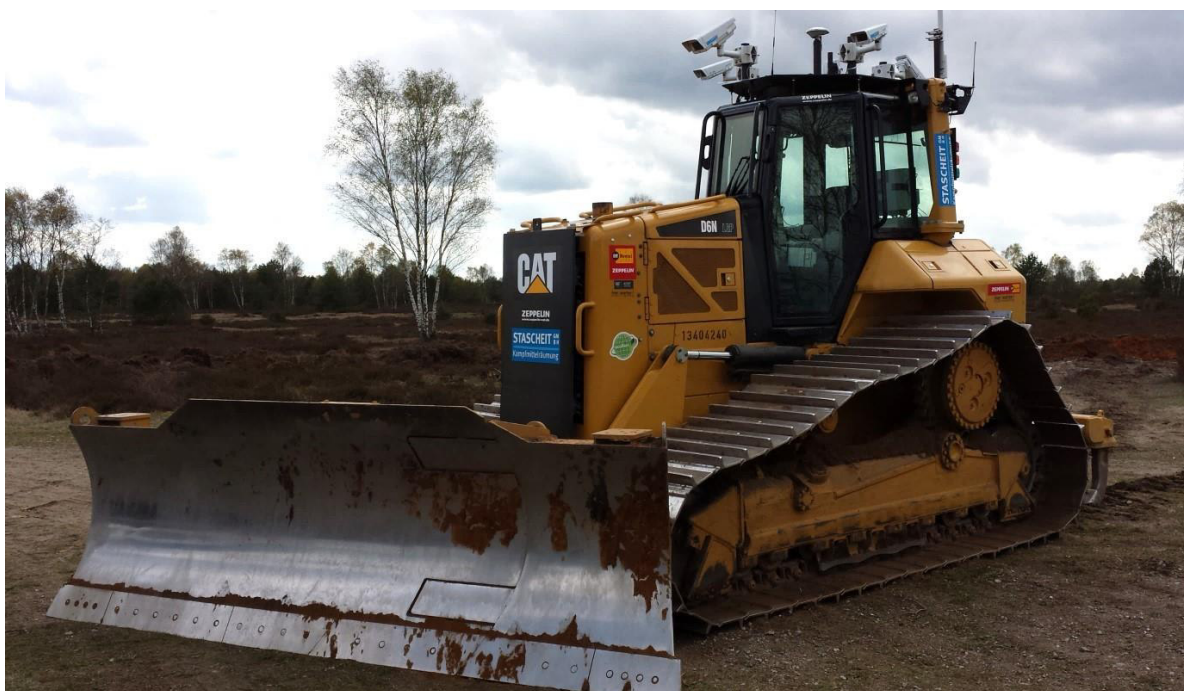
Figure 9: Unmanned, remote-controlled caterpillar used to create the firebreaks for the fire containment system. For further explanations, see text.
