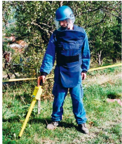
33 A sub-surface instrument search being conducted in Kosovo
