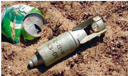
8 The Russian AO-1SCh is a simple fragmentation submunition
